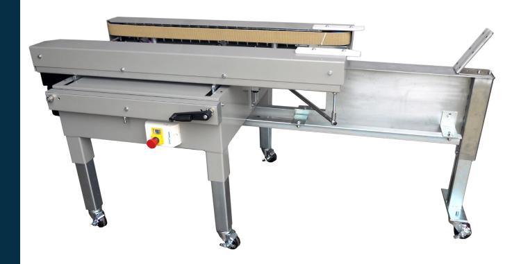
The SP-22V semi-automatic case erector and sealer closes the bottom four flaps of a corrugated case and seals it with tape. In one continuous motion, the operator squares a case and places it on the pack table (closing the minor bottom flaps). Then, the case is pushed to the side belts where the major flaps are automatically closed. Lastly, the pressure sensitive tape is applied from the bottom tape head.
