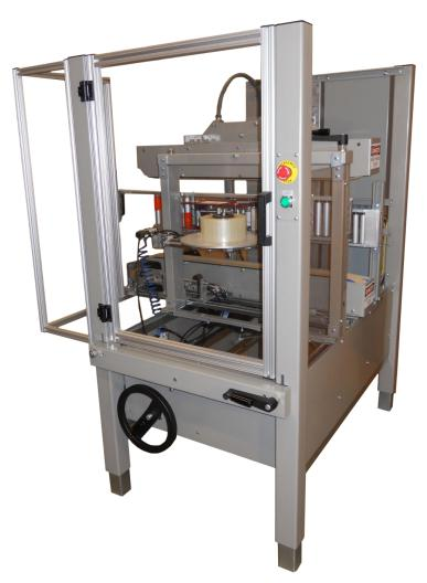
The SP-32 ST-S-E is compact machine designed to seal the edge of a corrugated box with tape. The machine can also seal the side of a box. It will work with a variatey of cartons such as RSC, FOL (full overlap carton), and POL (partial overlap carton). Exclusive features of the machine are interlocked safety guarding, welded frame with adjustable legs, and open face, custom built Sam Packaging tape head.
