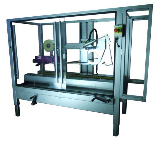
The SP-32TFC Automatic Case Sealer automatically closes the top case flaps and seals them with tape. Exclusive features of the machine are interlocked safety guarding, welded frame with adjustable legs, and open face, custom built Sam Packaging tape heads.
