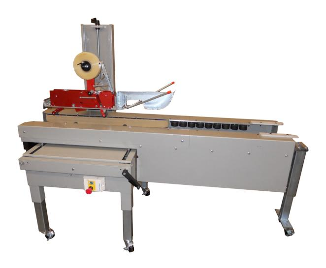
The SP-33 Econopack is a semiautomatic case pack and seal system with integrated pack station. Exclusive features of the machine are the pack station for "hands-free" case loading, welded frame with adjustable legs, and open face Sam Packaging tape heads.
