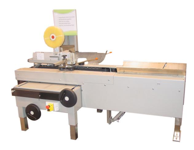
The SP-33PS is a semi-automatic case erect / pack / top and bottom case seal system with integrated pack station. Exclusive features of the machine are the pack station for "hands-free" case loading, welded frame with adjustable legs, and open face, custom built Sam Packaging tape heads.
